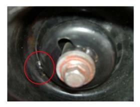
2) 在安裝 BC 避震器前,請先查看後車體兩側,在彈簧 調整上座跟車體連接處,確認焊接突出點之位置。 Before fitting the rear spring adjuster, check inside the rear cross member of the vehicle and spot the protrusion of the welding point around the upper mounting area. See (Pic 1 & 2)
